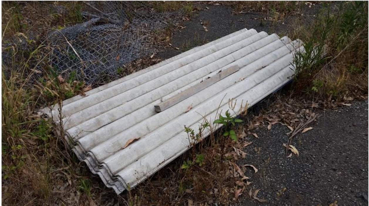
Photo 3: Super-six asbestos sheeting located within the grassed / gravelled area in the northern portion of the site.
